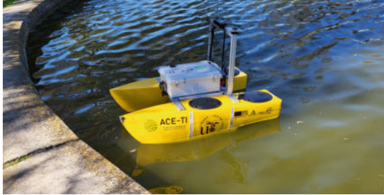
Fig. 1. Real ASV prototype proposed for WQP monitorization.
